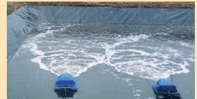
Turbo-Jet 1.1 kW floating – parallel operation
