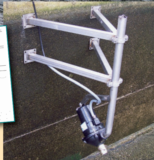
Turbo-Jet stationary 1.1 kW
